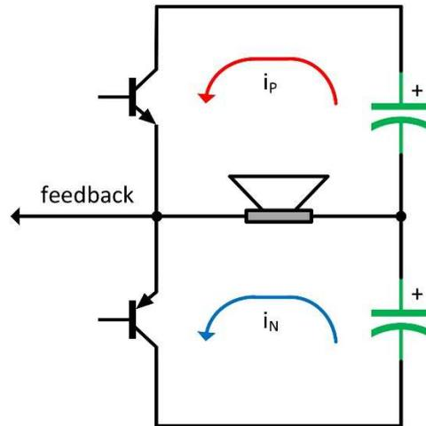
Figure 1. The amplifier output stage works in conjunction with the power supply
